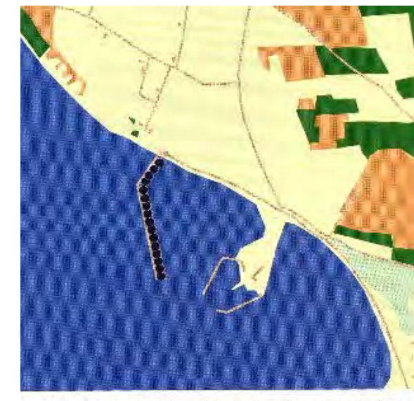
5. Ebeltoft, 16 galvanised Nordtank tube tower turbines, 55 kW, 1985, hub: 22 m, dia: 16 m. Perpendicular to the coast, pier construction related to harbour, short turbine spacing.
