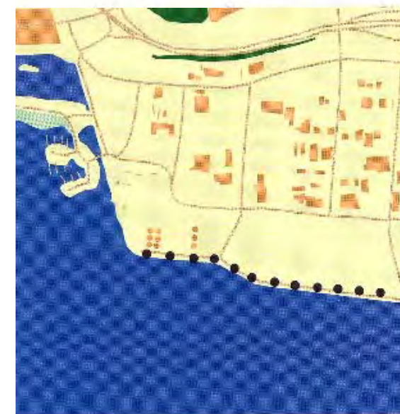
1. Avedøre, 12 Bonus tube tower turbines, 300 kW, 1992-93, hub: 33.5 m, dia: 31 m. Follows the coastline, connected to Avedøre power station, industrial features.
