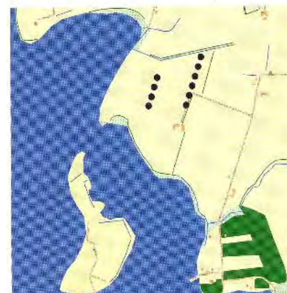
17. Oddesund, 25 Bonus tripod wind turbines, 95 kW, 1985-86, hub: 24 m, dia: 19.4 m. Broken row system, railway and high-tension transmission line.
