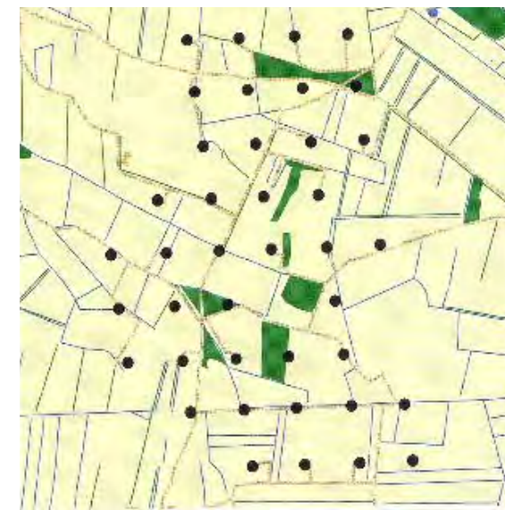
19. Røjsby, 10 Micon tube tower turbines, 600 kW, 1995, hub: 15 m, dia: 38 m. DK's most recent & most powerful wind farm, tight quadratic network, independent of roads and vegetation, flat terrain.
