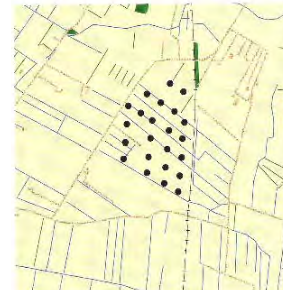
1. Avedøre, 12 Bonus tube tower turbines, 300 kW, 1992-93, hub: 33.5 m, dia: 31 m. Follows the coastline, connected to Avedøre power station, industrial features.
